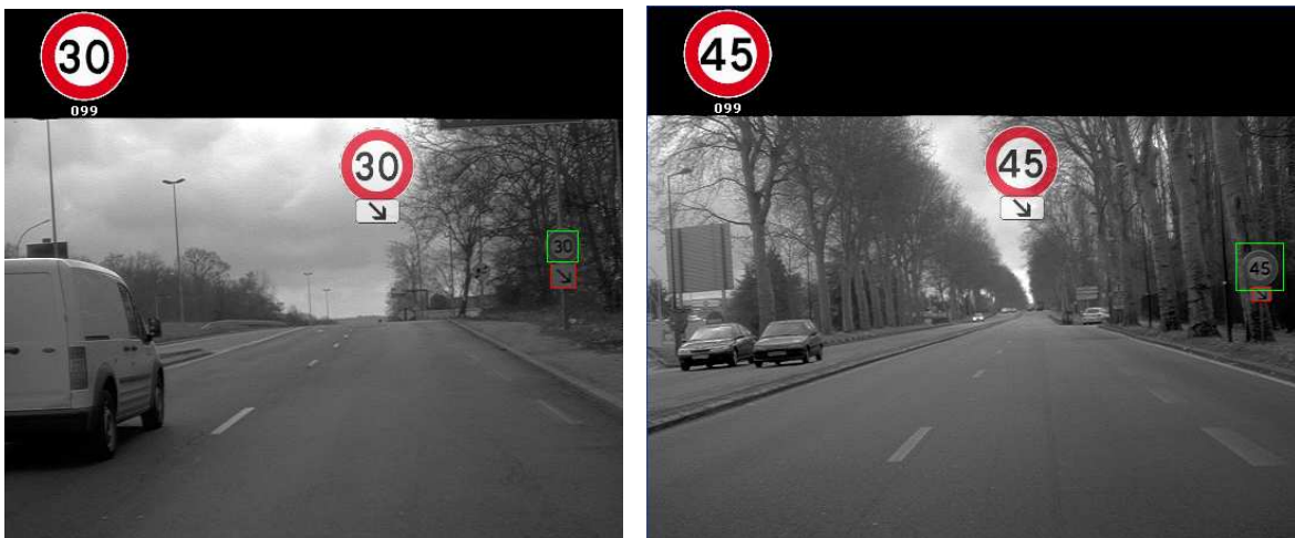
Fig. 4. Illustration of correct detection and recognition of square and big (left) as well as rectangular and small (right) French exit-lane supplementary signs
