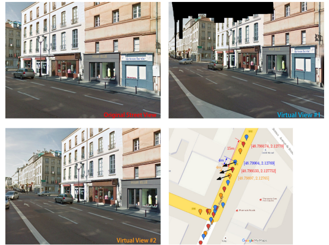
Fig. 5. Illustration of virtual views synthesized and back-projected from the original Street View panorama at location [48.799133, 2.127752]. The location of the rectilinear Street View, and the 4m forward and backward virtual views are colored respectively in red, orange and blue. The black arrows indicate the virtual camera view directions. Missing depth information causes null pixels in the virtual view #1.
