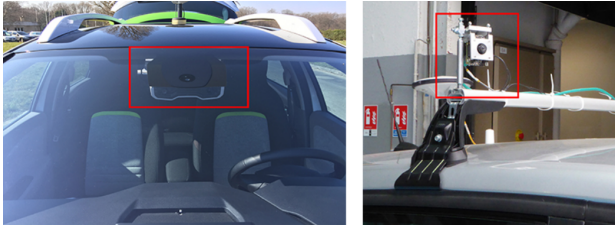
Fig. 4: Position of the cameras in the vehicle used in the experiments.
