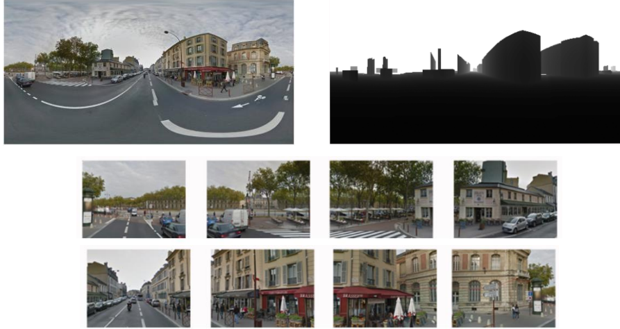
Fig. 2. On top, example of StreetView 360° panorama (upper-left) and its associated depth map (upper-right). On bottom, examples of generated rectilinear images with various orientations of viewpoint from the same point O (center of the source panorama).
