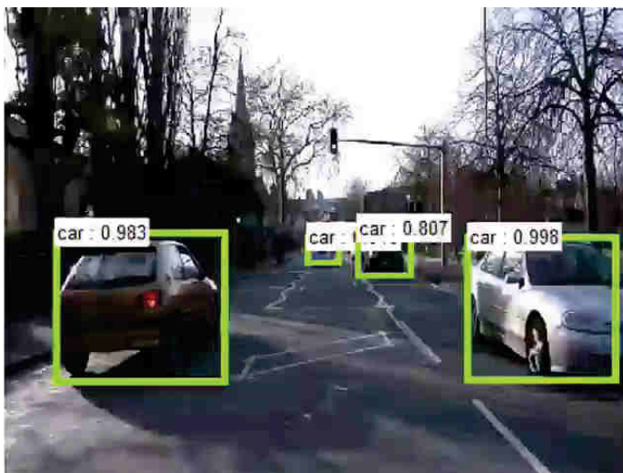
From camera (Visual object detection by Faster_RCNN)
